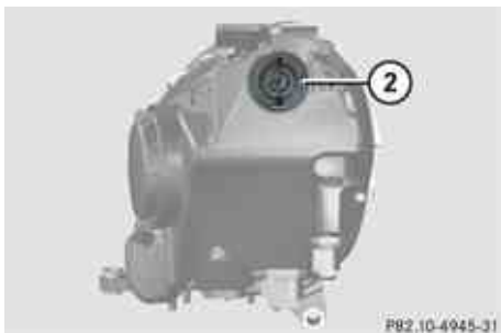
② Bulb socket for front turn signal lamp bulb
