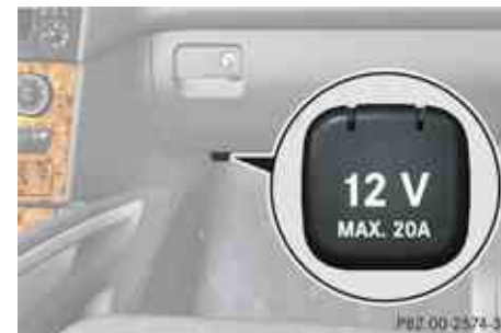
Power outlet in front passenger footwell
