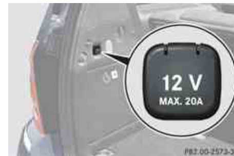
Power outlet in cargo compartment
