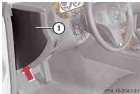
① Fuse box cover
