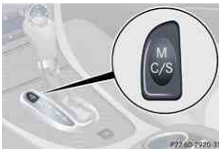
Program mode selector switch on CLK 63 AMG
