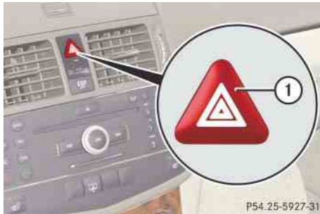
① Hazard warning flasher switch
