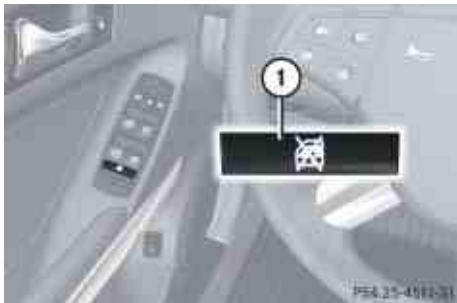
① Override switch
