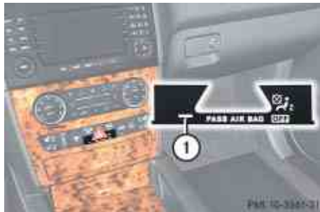
① Alarm system indicator lamp
