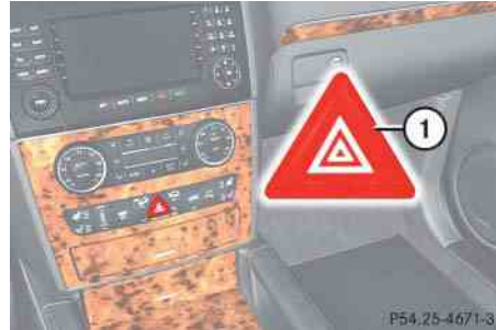
① Hazard warning flasher switch
