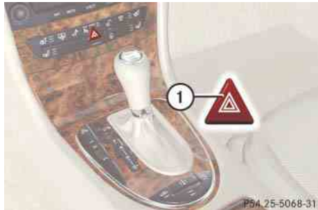
① Hazard warning flasher switch
