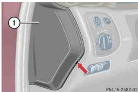
① Main fuse box cover
