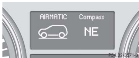
Example for compass display on vehicles equipped with AIRMATIC*
