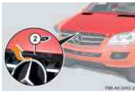
② Handle for opening the hood
