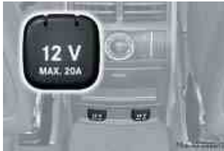
Power outlet in rear passenger footwell
