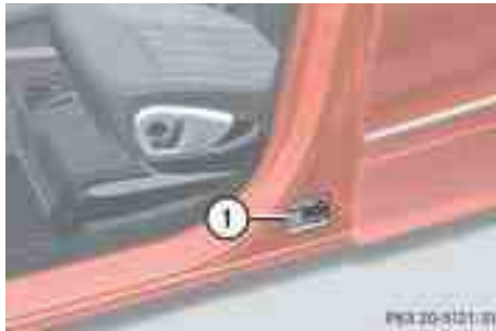
① Certification label (on driver's B pillar)
