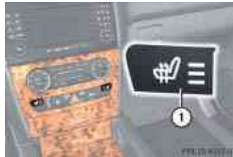
① Seat heating switch
