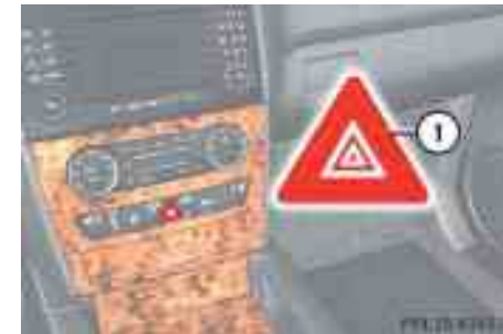
① Hazard warning flasher switch
