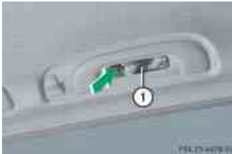
① Rear interior reading lamp
