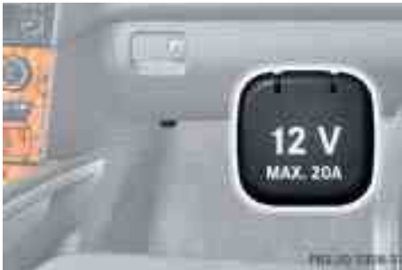
Power outlet in front passenger footwell
