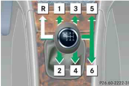
Gearshift pattern for manual transmission
