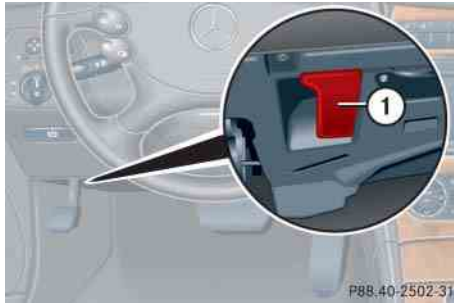
① Hood lock release lever
