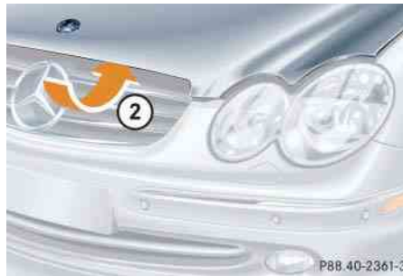
② Lever for opening the hood
