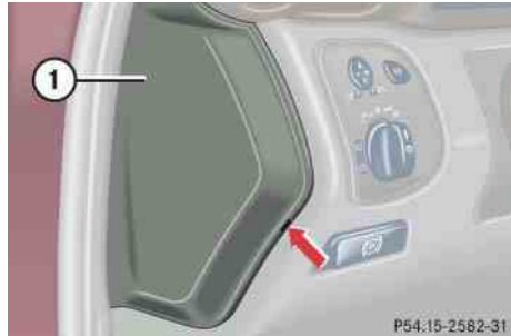
① Main fuse box cover
