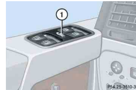
① Override switch
