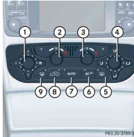
Climate control panel
