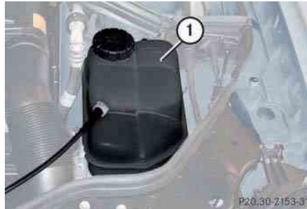
1 Coolant expansion tank
