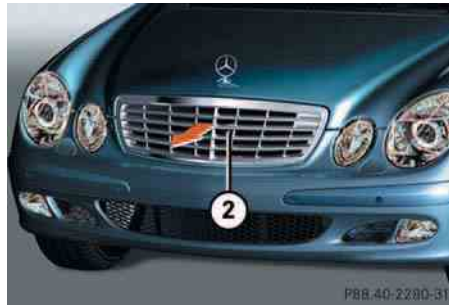
2 Handle for opening the hood
