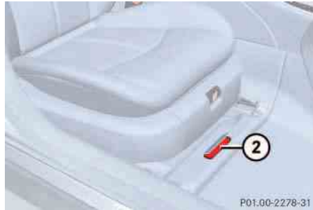
2 Vehicle Identification Number (VIN)
