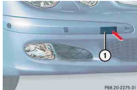
1 Cover on right side of front bumper
