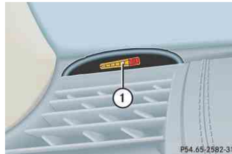
1 Left front area warning indicator
