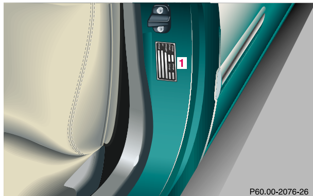
1 Certification label (below driver's door lock latch)
