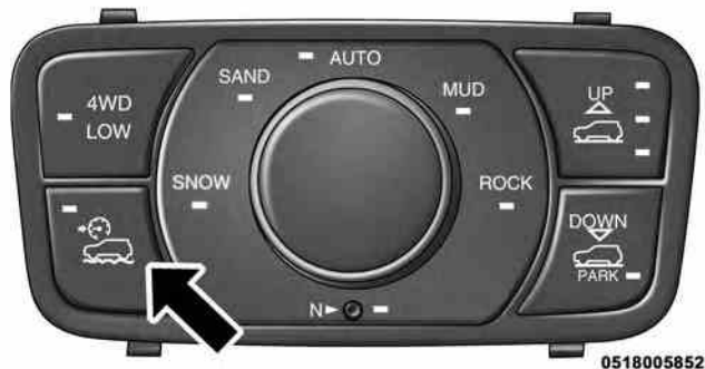
Select Speed Control Switch
