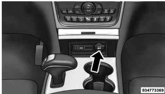
Front Power Outlet
