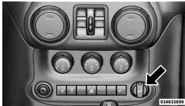
Front Power Outlet
