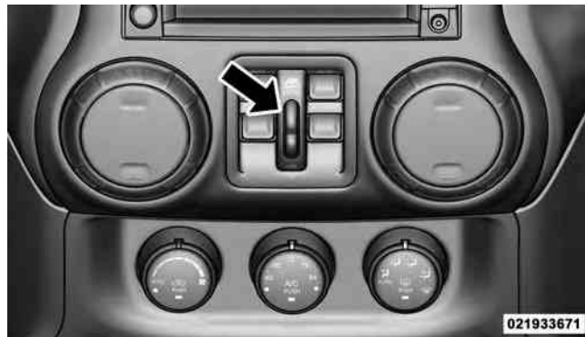
Window Lockout Switch
