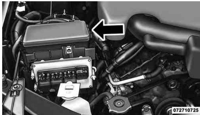
Totally Integrated Power Module
