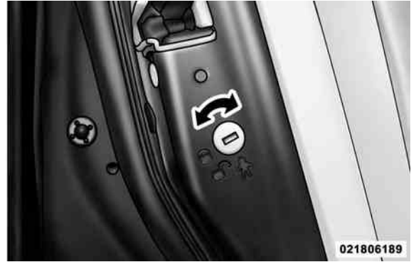
Child-Protection Door Lock Function
