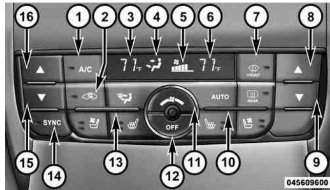
Automatic Temperature Control (ATC) Panel
