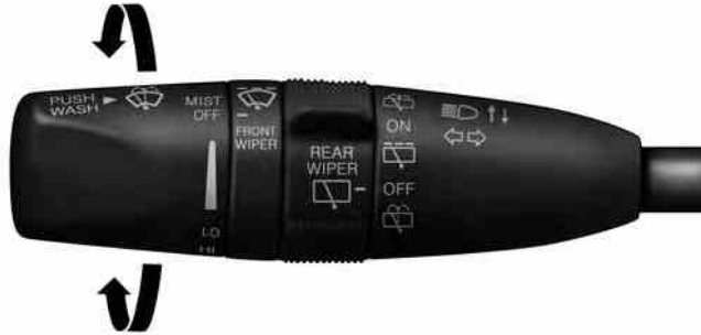
Windshield Wiper Operation
