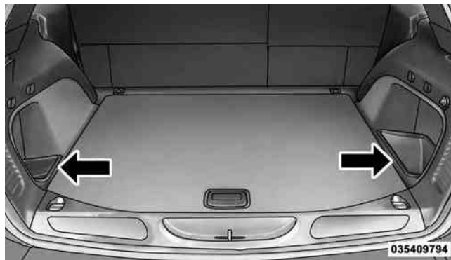
Rear Storage Bins
