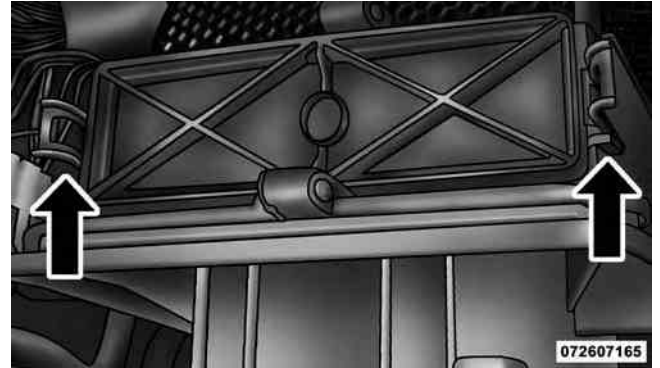
A/C Air Filter Replacement
