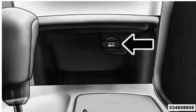
Front Power Outlet
