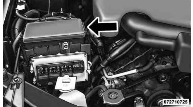
Totally Integrated Power Module
