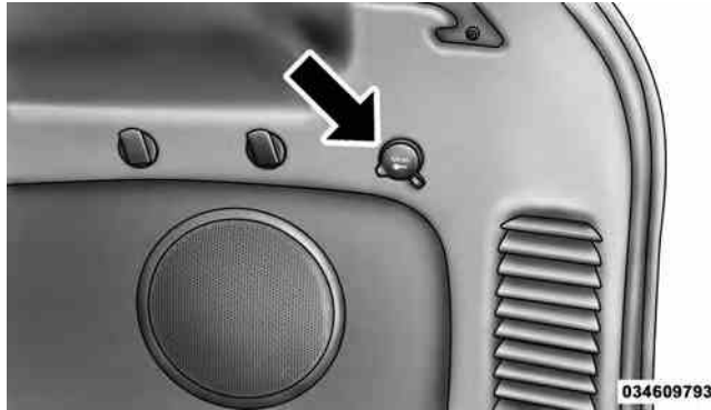
Rear Power Outlet
