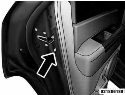
Child-Protection Door Lock Location
