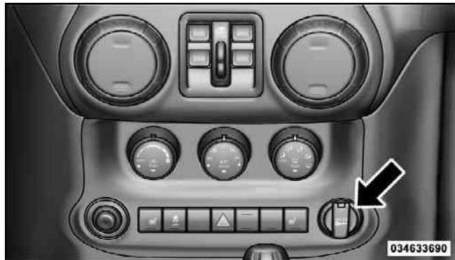
Front Power Outlet
