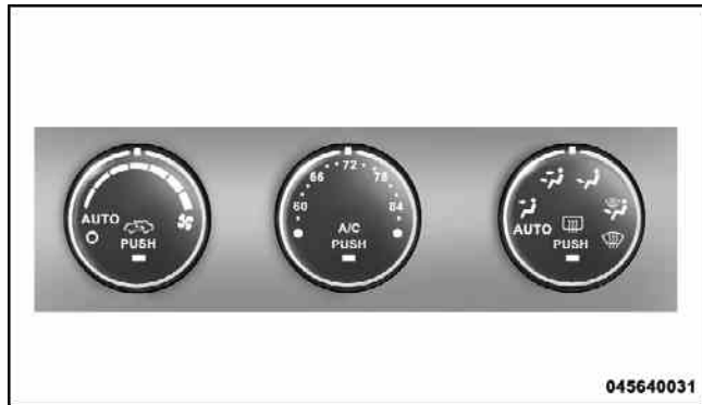
Automatic Temperature Control
