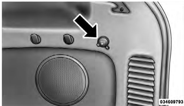
Rear Power Outlet
