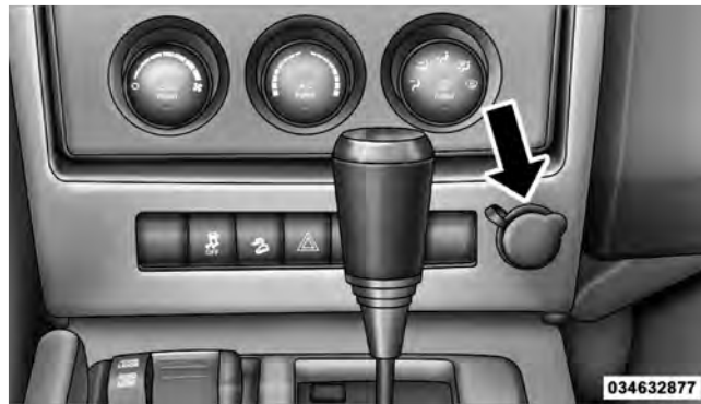
Front Power Outlet
