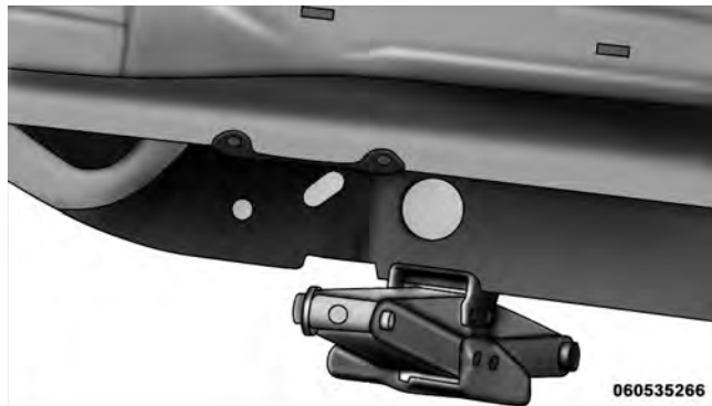
Front Jacking Location
