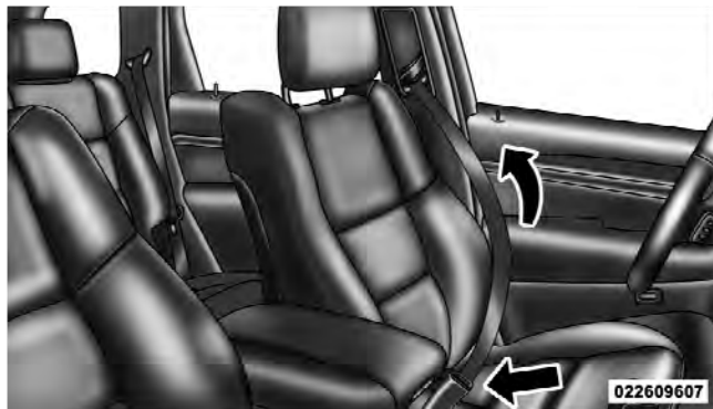
Removing Slack from Belt
