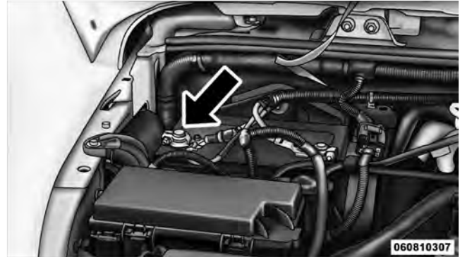
Positive Battery Post
