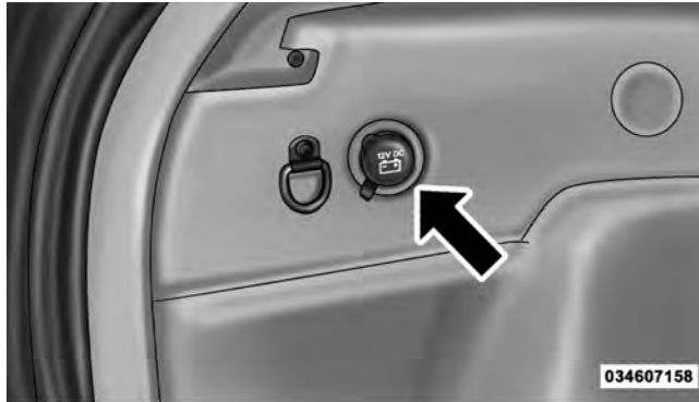
Rear Power Outlet
