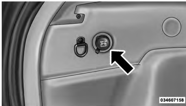
Rear Power Outlet
