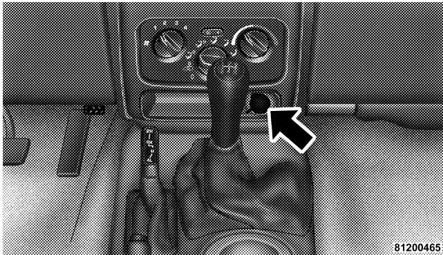
Front Power Outlet
