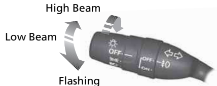
Light Control Switches
