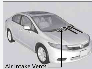
Air Intake Vents
