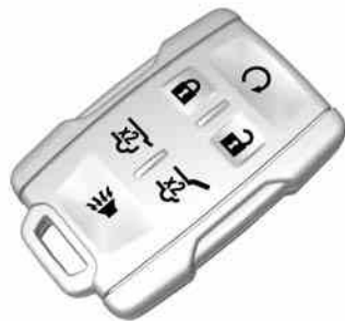
Key Access RKE Transmitter with Remote Start
