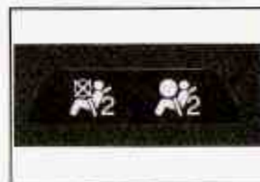
Passenger Air Bag Status Indicator – Canada
