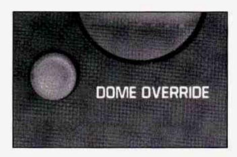
You can use the DOME OVERRIDE button, located below the parking/headlamp knob, to set the dome lamps to come on automatically when the doors are opened, or remain off. To turn the lamps off, press the button once. With the button in this position, the dome lamps will remain off when the doors are open. To return the lamps to automatic operation, press the button again and return it to the "out" position. With the button in this position, the dome lamps will come on when you open the door.
