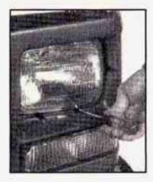
Remove the four screws from the headlamp retainer.
