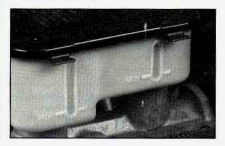
You can check the brake fluid without taking off the cap.
