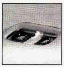
If your vehicle has reading lamps, press the button next to the lamp to turn the lamp on. The lamps can be adjusted to point in the direction you want.
