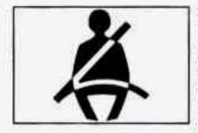
The safety belt light will also come on and stay on for about 20 seconds, then it will flash for about 55 seconds. If the driver's belt is already buckled, neither the tone nor the light will come on.
