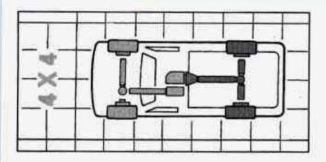
The front axle portion of the indicator diagram will light up when you shift into four-wheel drive and the front axle engages.
