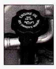
The engine oil fill cap for the "VORTEC" 4300, 5000 and 5700 engines are located on the driver's side engine valve cover.
