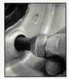
Replace the wheel nuts with the rounded end of the nuts toward the wheel. Tighten each wheel nut by hand using the wheel wrench until the wheel is held against the hub.
