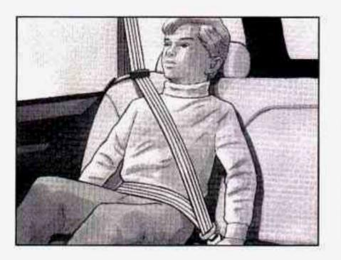
Buckle, position and release the safety belt as described in "Rear Seat Outside Passenger Positions (Extended Cab)" or "Rear Seat Outside Passenger Positions (Crew Cab)" earlier in this section. Make sure that the shoulder belt crosses the shoulder. To remove and store the comfort guides, squeeze the belt edges together so that you can take them out from the guides. Slide the guide onto the storage clip.
