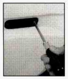
Remove the screws and take the fender marker assembly out of the fender.
