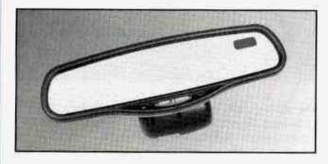
The mirror also includes an eight-point compass display in the upper right corner of the mirror face. When on, the compass automatically calibrates as the vehicle is driven.
