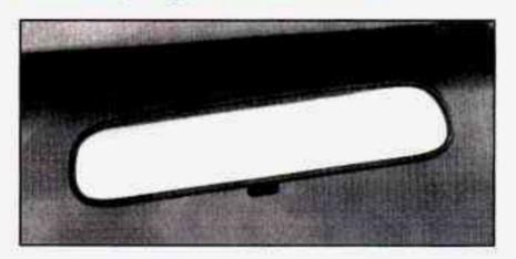
Pull the tab under the mirror rearward to reduce glare from headlamps behind you after dark. Push the tab forward for normal daytime operation.
