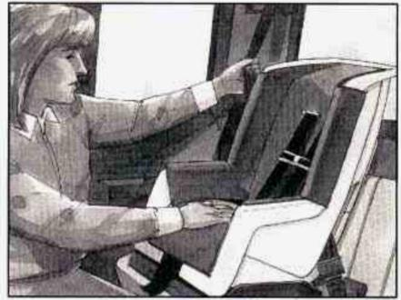
To tighten the belt, pull up on the shoulder belt while you push down on the child restraint. If you're using a forward-facing child restraint, you may find it helpful to use your knee to push down on the child restraint as you tighten the belt.
