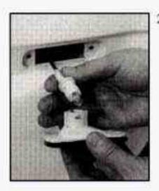
Turn the bulb socket to the left and remove it from the lens assembly.
