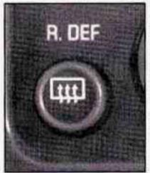
To turn on the rear window defogger, press this button next to the fan control knob. The rear window defogger will only work if the ignition switch is turned to RUN. For best results, clear the window of as much snow or ice as possible first.
