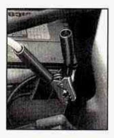
Now connect the black negative (-) cable to the good battery's negative (-) cable.
