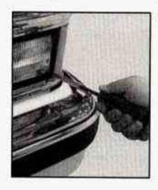
Remove the four screws and take out the parking/turn signal lamp assembly.
