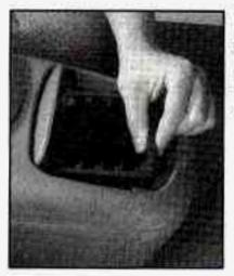
The cassette/compact disc holder can be removed and replaced with a cupholder that is located in the center console storage area.
