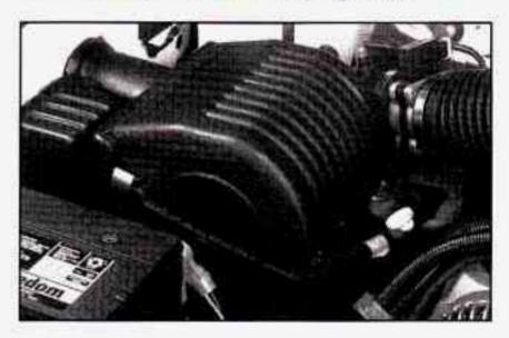
Your air cleaner is located between the battery and coolant recovery tank.
