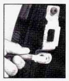
Raise the tailgate slightly and release both retaining cable clips. To release the retaining cable clips, pull the retaining cable clip away from the cable end. Lift the cable so it points straight out and push the cable clips forward.
