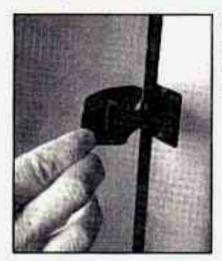
To open a rear swing-out window, just flip the latch open and swing the glass out.
