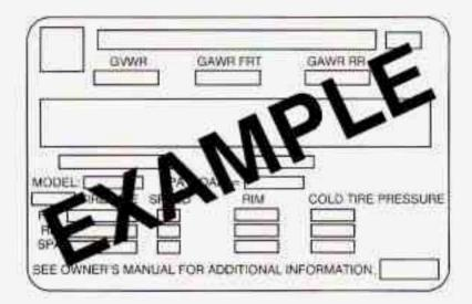
The Certification/Tire label is found on the rear edge of the driver's door or in the Incomplete Vehicle Document in the cab.
