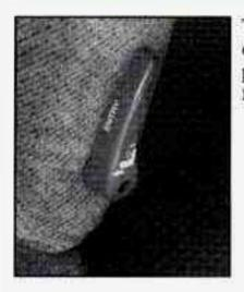
To fold a front split bench or bucket seatback forward, pull this lever forward and fold the seatback forward.
