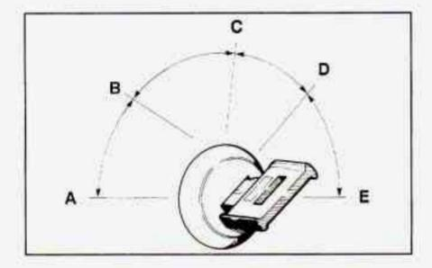
ACCESSORY (A): ACCESSORY lets you use things like the radio, power windows and the windshield wipers when the engine is off. Push in the key and turn it toward you. Your steering wheel will remain locked, just as it was before you inserted the key. LOCK (B): This position locks your ignition, steering wheel and transmission. It's a theft-deterrent feature. You will only be able to remove your key when the ignition is turned to LOCK.
