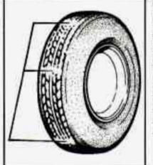
One way to tell when it's time for new tires is to check the treadwear indicators, which will appear when your tires have only 1/16 inch (1.6 mm) or less of tread remaining. Some commercial truck tires may not have treadwear indicators.
