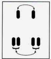
If your vehicle has dual rear wheels and the load range or tread design for your front tires is different from your rear tires, always use the correct rotation pattern shown here when rotating your tires. The dual tires are rotated as a pair, and the inside rear tires become the outside rear tires.
