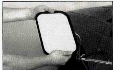
To adjust the mirrors when hauling a slide-in camper or towing a trailer, rotate the mirror by pushing the mirror head toward the front of the vehicle.
