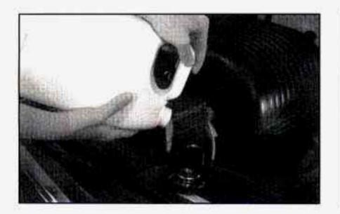
Fill the radiator with the proper DEX-COOL<sup>®</sup>
