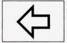
An arrow on the instrument panel will flash in the direction of the turn or lane change.
