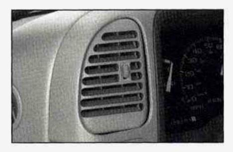
Your vehicle has air outlets in the center and on the sides of your instrument panel. You can move the outlets from side-to-side or up and down to direct the flow of air, or close the outlets altogether. When you close an outlet, it will increase the flow of air coming out of any outlets that are open. These outlets do not completely shut off airflow when in the closed position.
