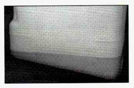
The coolant level should be at or above the COLD mark.
