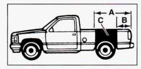
Use the rear edge of the load floor for measurement purposes. The recommended location for the cargo center of gravity is at point C for the CWR. It is the point where the mass of a body is concentrated and, if suspended at that point, would balance the front and rear. Here is an example of proper truck and camper match:
