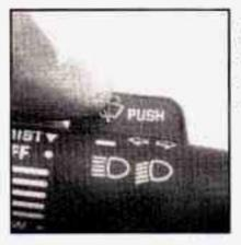
At the top of the lever, there's a paddle with the word PUSH on it. To spray washer fluid on the windshield, push the paddle.
