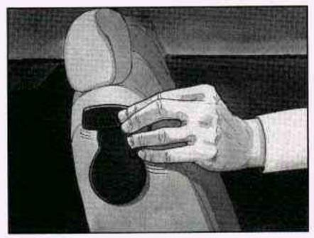
Remove the guide from its storage clip on the side of the seatback.
