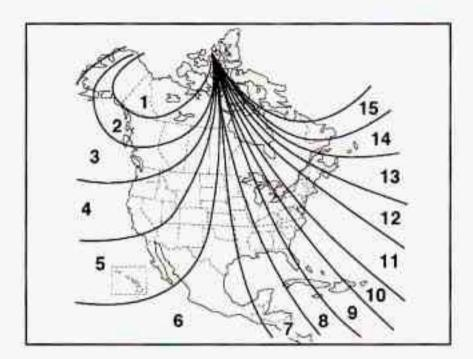
Press the COMP button on the bottom of the mirror until the new zone number appears in the display.
