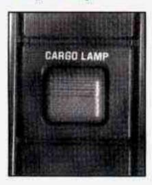
Press the ribbed top part of the switch to turn the cargo lamp on. Press the bottom of the switch to turn it off.
