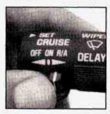
Once you're going about 25 mph (40 km/h) or more, you can move the cruise switch from ON to R/A (Resume/Accelerate) for about half a second.
