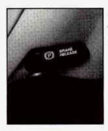
Pull the lever, located just above the parking brake pedal, marked BRAKE RELEASE.
