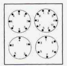
8. Tighten the nuts firmly in a crisscross sequence as shown by rotating the wheel wrench to the right.
