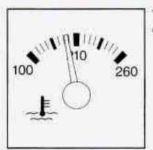
This gage shows the engine coolant temperature. It also provides an indicator of how hard your vehicle is working. During a majority of the operation, the gage will read 210°F (100°C) or less. If you are pulling a load or going up hills, it is normal for the temperature to fluctuate and approach the 260°F (125°C) mark. If the gage reaches the 260°F (125°C) mark, it indicates that the cooling system is working beyond its capacity.
