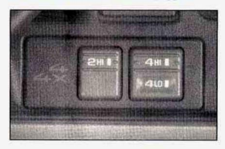
If your four-wheel-drive vehicle has the electronic transfer case, the transfer case switches are below and to the left of the climate control system. Use these switches to shift into and out of four-wheel drive. You can choose among three driving settings:
