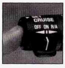
Press in the SET button at the end of the lever and release it.
