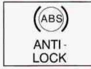
With the anti-lock brake system, this light will come on when you start your engine and may stay on for several seconds. That's normal.
