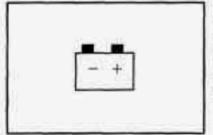
This light should come on briefly when you turn on the ignition, before starting the engine, as a check to show you it is working.
