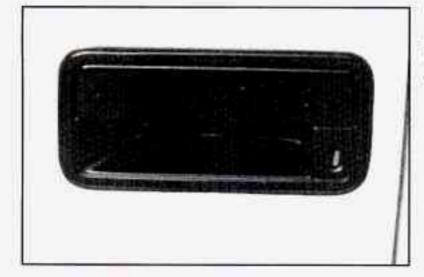
To open the door from the outside, pull the handle up and pull the door open.
