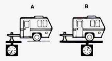
If you're using a "dead-weight" hitch, the trailer tongue (A) should weigh 10% of the total loaded trailer weight (B). If you have a "weight-distributing" hitch, the trailer tongue (A) should weigh 12% of the total loaded trailer weight (B).
