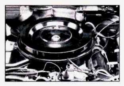
To remove the air cleaner filter on a gas engine or a 6.5 liter naturally aspirated diesel, turn the wing nuts to the left. Remove the cover and change the filter.
