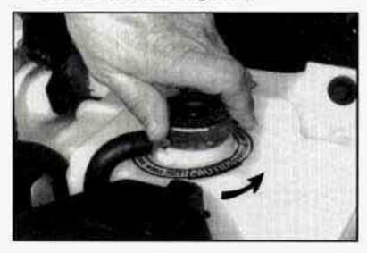
Turn the pressure cap slowly to the left until it first stops. (Don't press down while turning the pressure cap.)
