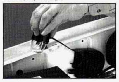
When you are done using the light, reel the cord back into the housing by turning the handle.
