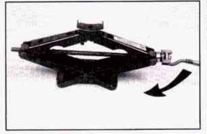
With the **UP** marking on the ratchet facing you, rotate the ratchet to the right.
