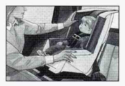
To remove the child restraint, just unbuckle the vehicle's safety belt and let it go back all the way. The safety belt will move freely again and be ready to work for an adult or larger child passenger.
