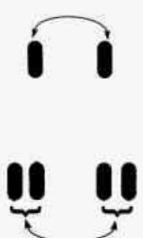
Use this pattern if your front and rear tires are different sizes or load ranges. The dual rear tires are rotated as a pair and the inside rear tires become the outside rear tires.
