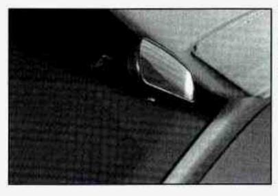
Push or pull the tab under the mirror to reduce glare from headlights behind you after dark.
