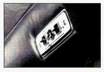
If your vehicle has a power seat on the driver's side, you can adjust it with this switch at the front of the seat.
