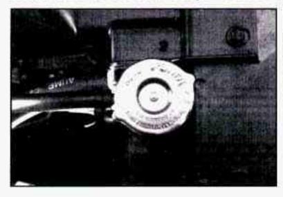
The radiator pressure cap must be tightly installed with the arrows on the cap lined up with the overflow tube on the radiator filler neck.
