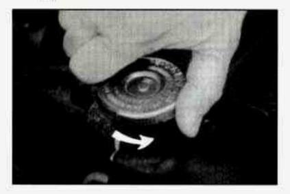
Turn the pressure cap slowly to the left until it first stops. (Don't press down while turning the pressure cap.)
