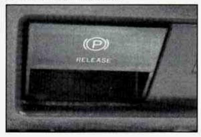
Hold the regular brake pedal down. Pull the lever, located just above the parking brake pedal, marked **RELEASE** to release the parking brake.
