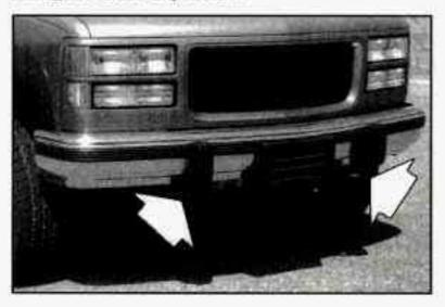
If you ever get stuck in sand, mud, ice or snow, your vehicle may be equipped with recovery hooks. The recovery hooks are provided at the front of your vehicle. You may need to use them if you're stuck off-road and need to be pulled to some place where you can continue driving.
