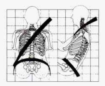
To make the lap part tight, pull down on the buckle end of the belt as you pull up on the shoulder part.
