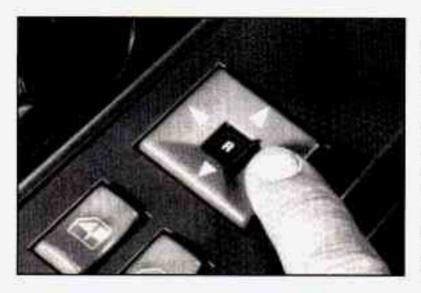
Select the mirror you want to move by moving the center of the switch, located on the driver's door armrest, to **R** (right) or **L** (left). Then, adjust the mirror angle by pressing the outer arrows on the switch until the mirror is adjusted where you want it.
