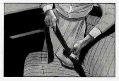
Make the belt as long as possible by tilting the latch plate and pulling it along the belt.
