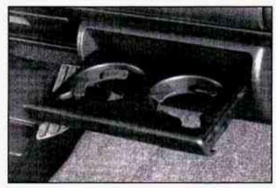
To use the cup holder, pull the handle and slide the cup holder tray out until it stops. Then, let the cup holder swing down into position.
