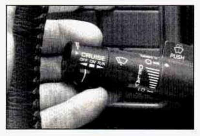
To change the headlights from low beam to high or high to low, pull the turn signal lever all the way toward you. Then release it.
