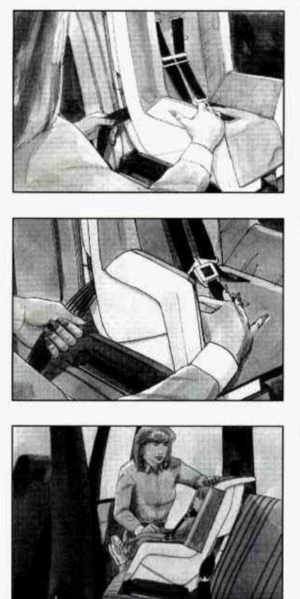
Pull the rest of the lap belt all the way out of the retractor to set the lock.
