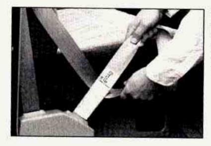
The model number on the replacement belt must be listed on the safety belt you want to replace. Pull the shoulder belt all the way out to see this label.
