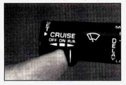
Move the Cruise switch from ON to R/A. Hold it there until you get up to the speed you want, and then release the switch.
