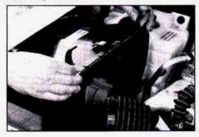
Then, unbook the cover retaining clips and push the rear of the cover toward the engine.
