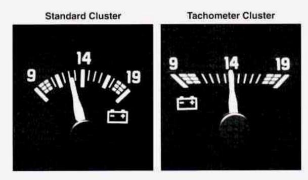
When your engine is not running, but the ignition is on (in the **RUN** Position), this gage shows your battery's state of charge in DC volts. When the engine is running, the gage shows the condition of the charging system. Readings between the low and high warning zones indicate the normal operating range.
