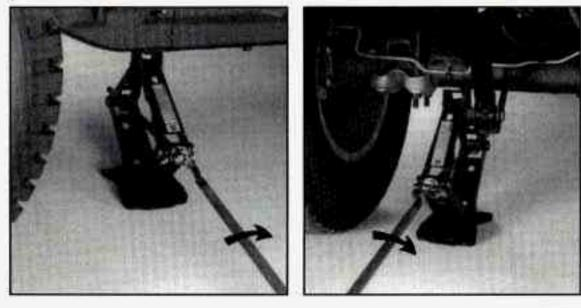
Raise the vehicle by rotating the ratchet to the right. Make sure the UP marking faces you. Use the jack handle extentions if the flat is on the rear of the vehicle. Raise the vehicle far enough off the ground so there is enough room for the spare tire to fit.
