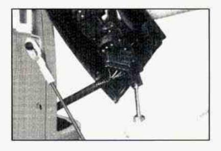
Remove the screws from the bulb retainer and take it off the light assembly.
