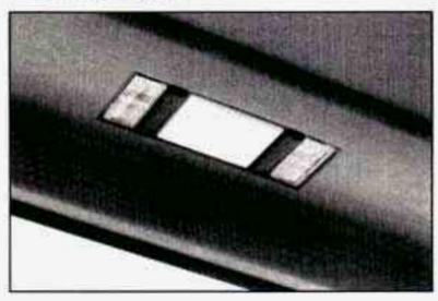
If your vehicle has reading lights, press the bar next to the light to turn the light on. Press the bar again to turn the light off.
