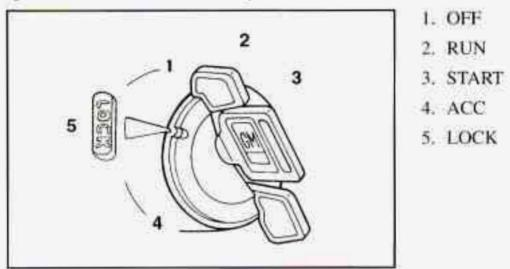
ACC (Accessory): ACC lets you use things like the radio and the windshield wipers when the engine is off. To get into ACC, push in the key and turn it toward you. Your steering wheel will remain locked, just as it was before you inserted the key.
