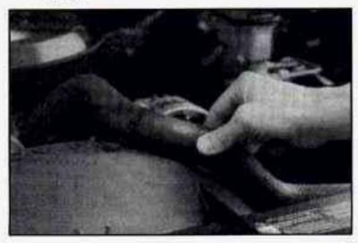
With the air bleed valve closed and the coolant surge tank pressure cap off, start the engine and let it run until you can feel the upper radiator hose getting hot.
