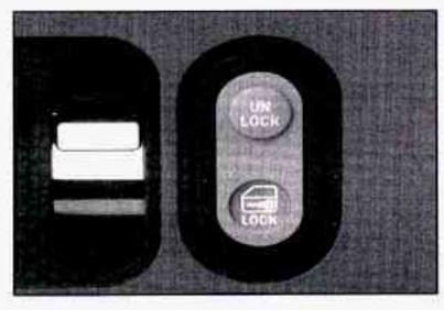
Press the bottom of the power door lock switch, marked LOCK, on either front door to lock all the doors at once. Press the switch marked UNLOCK to unlock all the doors at once.
