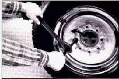
Using the wheel wrench and ratchet, with **DOWN** facing you, loosen all the wheel nuts.
