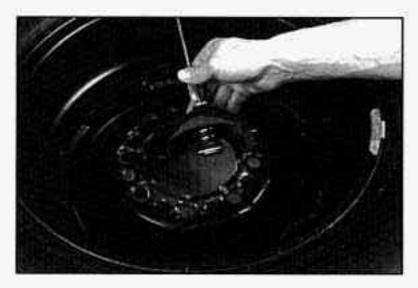
When the tire has been lowered, tilt the retainer at the end of the cable and pull it through the wheel opening.
