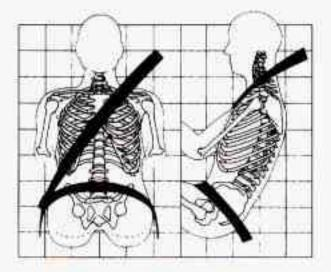
The driver has a lap-shoulder belt. Here's how to wear it properly.
