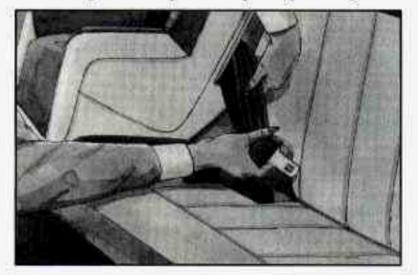
4. Run the lap and shoulder portions through or around the restraint. The child restraint instructions will show you how. If the shoulder belt goes in front of the child's face or neck, put it behind the child restraint.
