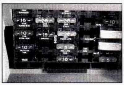
The fuse block is behind an access door at the bottom of the instrument panel, next to the parking brake release lever.
