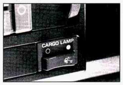
To turn your optional cargo lamp on, push the side of the switch with the cargo lamp symbol on it.
