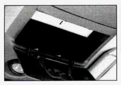
Peel the protective backing from the hook and loop patch. Press it firmly to the back of your garage door opener, as close to the center of the opener as possible.
