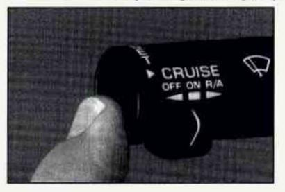
Push the button at the end of the lever, then release the button and the accelerator pedal. You'll now cruise at the higher speed. Here's the second way to go to a higher speed:
