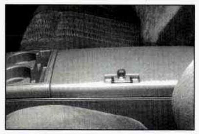
To open it, just squeeze the buttons on both sides of the keyhole, and pull up. Use your round key to lock this compartment.
