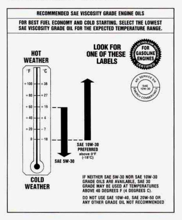
As shown in the chart, SAE 10W-30 is best for your vehicle. However, you can use SAE 5W-30 if it's going to be colder than 60°F (16°C) before your next oil change. When it's very cold, you should use SAE 5W-30. These numbers on an oil container show its viscosity, or thickness. Do not use other viscosity oils, such as SAE 10W-40 or SAE 20W-50.
