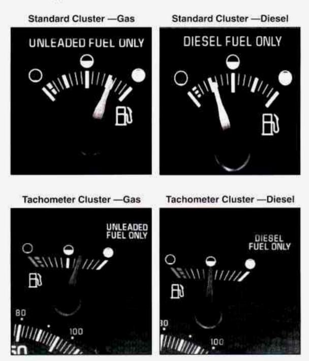
The fuel gage, when the ignition is on, tells you about how much fuel you have left in your tank. The gage will first indicate empty before you are out of fuel, and you should get more fuel as soon as possible.
