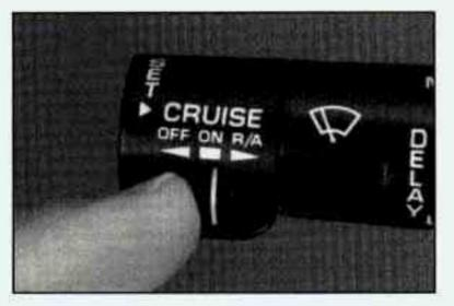
Move the Cruise Control switch to ON.
