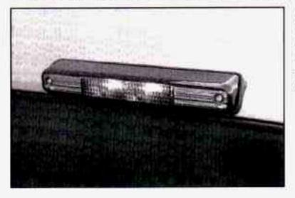
Your vehicle may have a Center High Mount Stop lamp (CHMSL) located above the rear window. If equipment such as a cap or camper is installed, a wire labeled "Center High Mount Stop lamp (CHMSL) feed" is provided along the left rear frame rail. This wire should be used to connect a CHMSL on the cap or camper.
