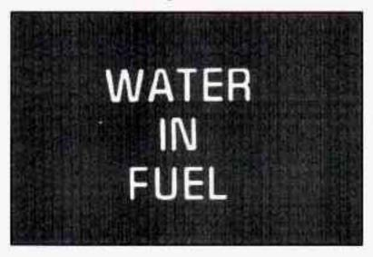
The red Water in Fuel light, if you have one, is located near the middle right edge of the instrument cluster, just below the turn signal and lane change indicator.
