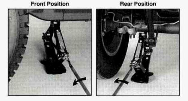
Lower the vehicle by rotating the ratchet to the left. Lower the jack completely.
