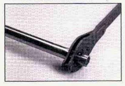
Attach the ratchet, with the **DOWN** marking facing you, to the wheel wrench.
