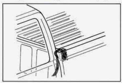
An optional 5-wire harness is stored in the front stake pocket on the driver's side of the bed. The harness has no connector, and should be wired by a qualified electrical technician.
