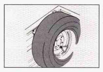
it may be mounted to the inside of the truck bed on the driver's side.
