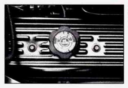
The engine oil filler cap is located on the driver's side engine valve cover.
