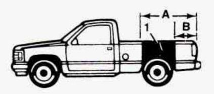
Recommended location for cargo center of gravity for cargo weight rating (Pickup Truck).
