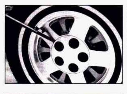
If the wheel has a smooth center piece or a center piece with recessed nuts, place the flat end of the wheel wrench in the slot on the wheel and pry out gently.
