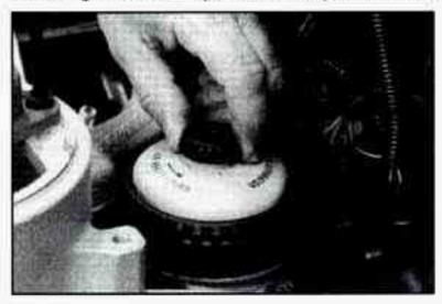
First, open the fuel filter air bleed valve. If there is air, then you are probably out of fuel.
