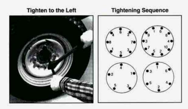
Tighten the nuts firmly in a criss-cross sequence as shown. Rotate the ratchet to the right with the UP marking facing you.
