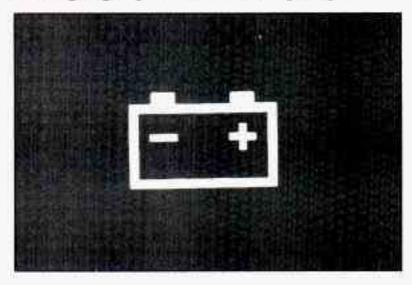
The red Charging System Warning light is located at the upper right corner of the instrument cluster.
