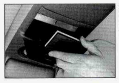
Center the garage door opener activation button over the console door button, and press the opener firmly into place.
