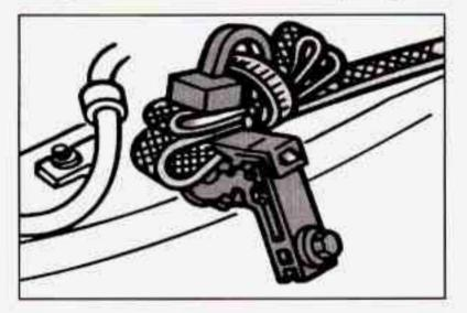
In very cold weather, 0°F (-18°C) or colder, the engine coolant heater can help. You'll get easier starting and better fuel economy during engine warm-up. Usually, the coolant heater should be plugged in a minimum of four hours prior to starting your vehicle. To use the coolant heater:
