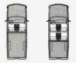
When you secure a child restraint in a center seating position, you'll be using the lap belt.
