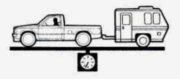
If your vehicle comes with the Trailering Package, there is also a load rating which includes the weight of the vehicle **and** the trailer it tows. This rating is called the Gross Combination Weight Rating (GCWR).
