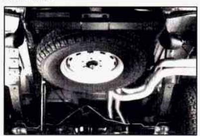
Your spare tire may be mounted underneath the rear of the vehicle, **OR**;
