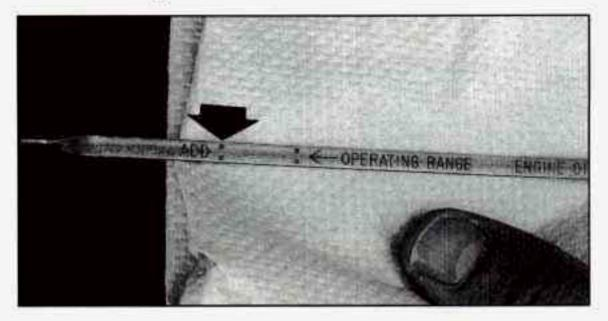
Pull out the dipstick and clean it with a paper towel or a cloth, then push it back in all the way. Remove it again, keeping the tip lower.
