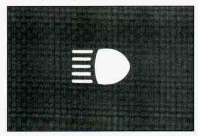
The blue Headlight High Beam Indicator light is located near the middle left edge of the instrument cluster.
