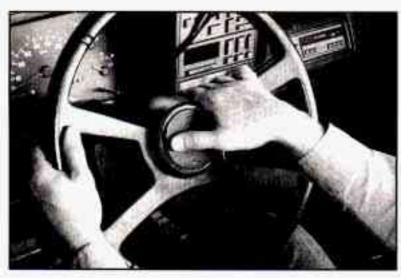
To sound the horn, press the pad in the center of the steering wheel. The pad has a horn symbol on it.
