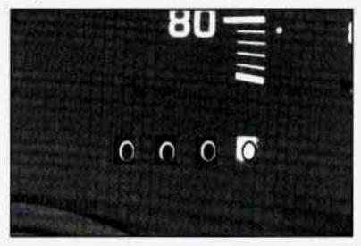
The trip odometer can tell you how far your vehicle has been driven since you last set the trip odometer to zero. To reset the trip odometer, fully press the reset button located near the trip odometer readout. If the reset button is not fully pressed, the trip odometer may not go all the way back to zero. If it doesn't, you may have to press the reset button again to reset the readout to zero.
