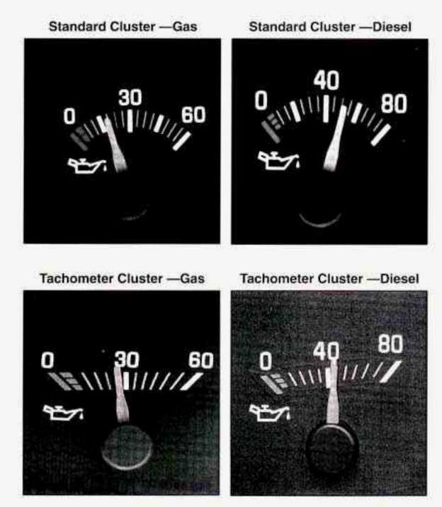
The oil pressure gage shows the engine oil pressure in psi (pounds per square inch) when the engine is running. Canadian vehicles indicate pressure in kPa (kilopascals). Oil pressure may vary with engine speed, outside temperature and oil viscosity, but readings above the low pressure zone indicate the normal operating range.
