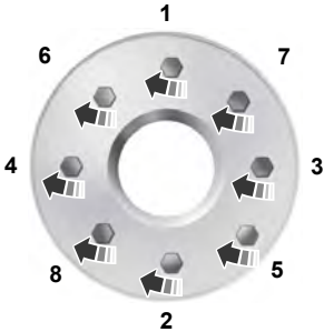
8-lug nut torque sequence
