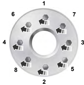
8-lug nut torque sequence
