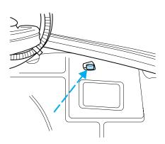
If your vehicle is a wagon, the fuel pump shut-off switch is located behind the service panel on the right side of the cargo area.
