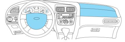
The airbag supplemental restraint system (SRS) is designed to work in conjunction with the safety belts to help protect the driver and front outboard passenger from certain upper body injuries. The term "supplemental restraint" means the airbags are intended as a supplement to the safety belts. Airbags alone cannot protect as well as airbags plus safety belts in impacts for which the airbags are designed to deploy, and airbags do not offer any protection in crashes for which they do not deploy.
