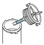
5. If the fluid is low, add fluid in small amounts, continuously checking the level until it reaches the FULL HOT range. Be sure to put the dipstick back in the reservoir.
