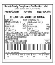
Exceeding the Safety Certification Label vehicle weight rating limits could result in substandard vehicle handling or performance, engine, transmission and/or structural damage, serious damage to the vehicle, loss of control and personal injury.
