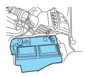
However, for severe usage or in high temperature climates, check the battery electrolyte level. Refer to *scheduled maintenance information* for the service interval schedules.
