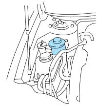
Check the power steering fluid. Refer to the *scheduled maintenance information* for the service interval schedules. If adding fluid is necessary, use only MERCON<sup>®</sup> ATF.
