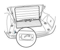
To close the seat, make sure the safety belts are properly stowed, then lift the remote latch release and push the seat down until it latches. Pull up on the handle and push the floor panel into place.
