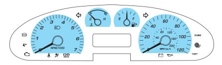
**Speedometer:** Indicates the current vehicle speed.
