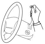
If your vehicle is equipped with a console-mounted gearshift lever, you must press the thumb button on the side of the gearshift lever to move the gearshift lever from P (Park).
