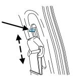
pull the control down and slide the height adjuster up. Pull down on the height adjuster to make sure it is locked in place.
