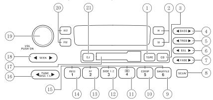
1. **Tape:** Insert the cassette with the opening to the right. If a tape is already inserted into the system, press TAPE to begin tape play.
