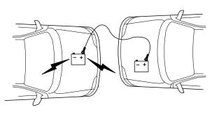
3. Remove the jumper cable from the positive (+) terminal of the booster vehicle's battery.
