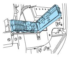
Always disconnect the battery before servicing high current fuses.
