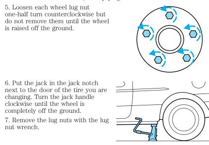
8. Replace the flat tire with the spare tire, making sure the valve stem is facing outward. Reinstall lug nuts until the wheel is snug against the hub. Do not fully tighten the lug nuts until the wheel has been lowered.
