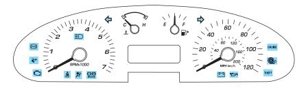
Warning lights and gauges can alert you to a vehicle condition that may become serious enough to cause expensive repairs. A warning light may illuminate when a problem exists with one of your vehicle's functions. Many lights will illuminate when you start your vehicle to make sure the bulb works. If any light remains on after starting the vehicle, have the respective system inspected immediately.
