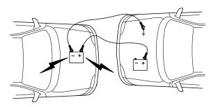
4. Make the final connection of the negative (-) cable. Make the connection to an exposed metal part of the stalled vehicle's engine, away from the battery and the carburetor/fuel injection system. **Do not** use fuel lines, engine rocker covers or the intake manifold as *grounding* points.
