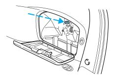
Use the following procedure to reset the fuel pump shut-off switch.
