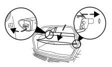
To reduce the risk of injuries, the fasteners for cargo area cover must be properly attached to the mounting clips on the rear trim panels.
