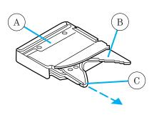
5. Line up the CD with the groove of the disc holder. Ensure that the label on the CD faces downwards.
