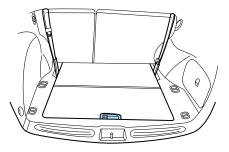
3. Lift the remote latch release on the left side of the compartment and fold the remaining floor panel until it latches. Make sure the seatback is locked in the upright position.
