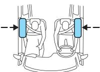
not of the type sufficient to cause activation. Side airbags are designed to inflate in side-impact collisions, not roll-over, rear-impact, frontal or near-frontal collisions, unless the collision causes sufficient lateral deceleration.
