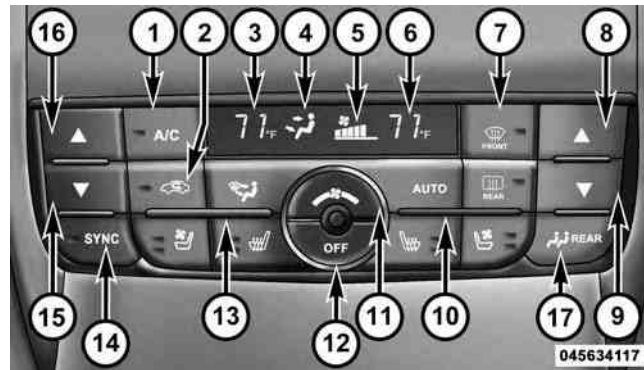
Automatic Temperature Control (ATC) Panel
