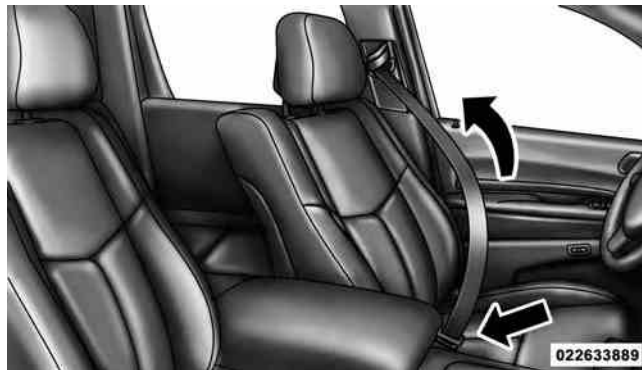
Removing Slack From Belt
