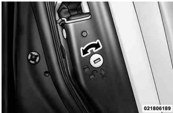
Child-Protection Door Lock Function
