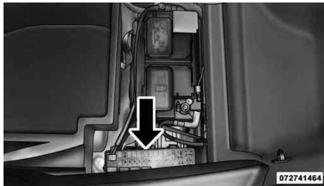
Rear Power Distribution Center
