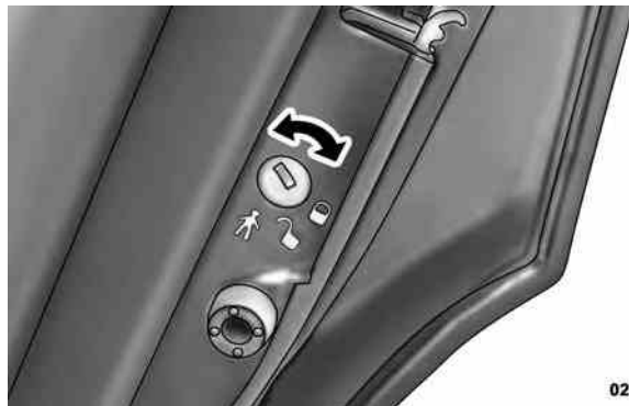
Child-Protection Door Lock Function
