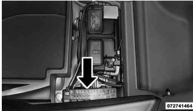
Rear Power Distribution Center
