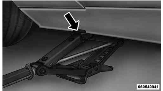
Front Jacking Location
