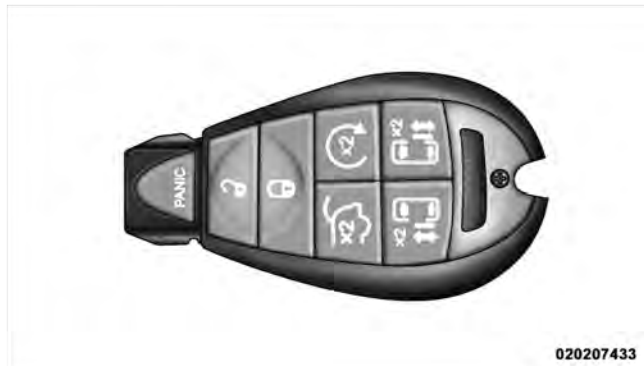
Key Fob With Seven-Button RKE Transmitter
