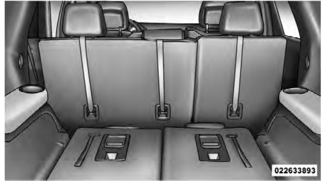
Top Tether Strap Mounting (60/40 Seat)
