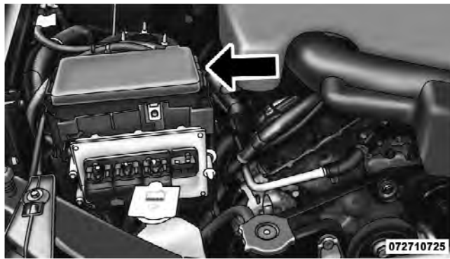
Totally Integrated Power Module
