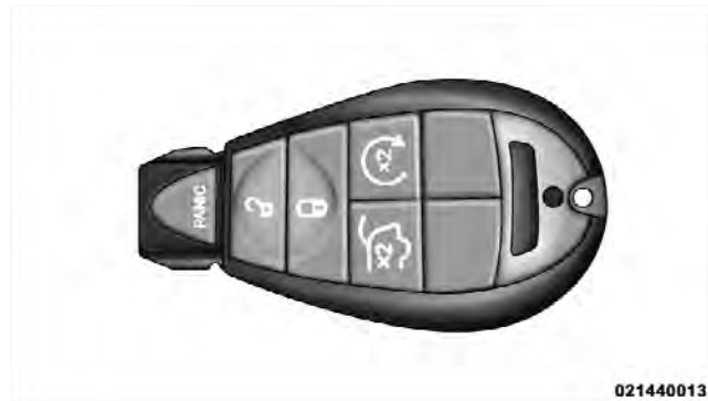
Key Fob With Five-Button RKE Transmitter
