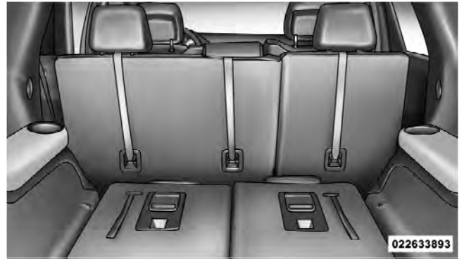
Top Tether Strap Mounting (60/40 Seat)
