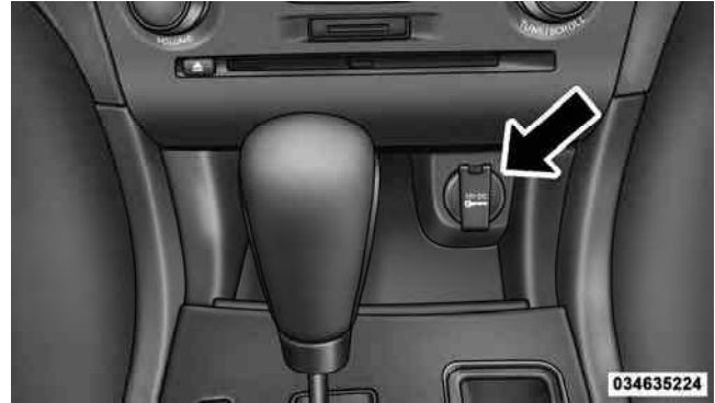
Front Power Outlet
