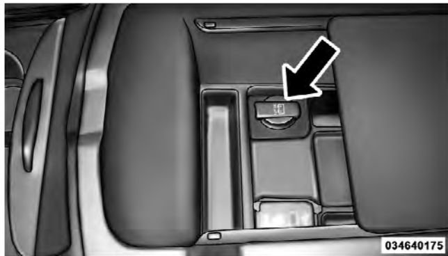
Center Console Power Outlet
