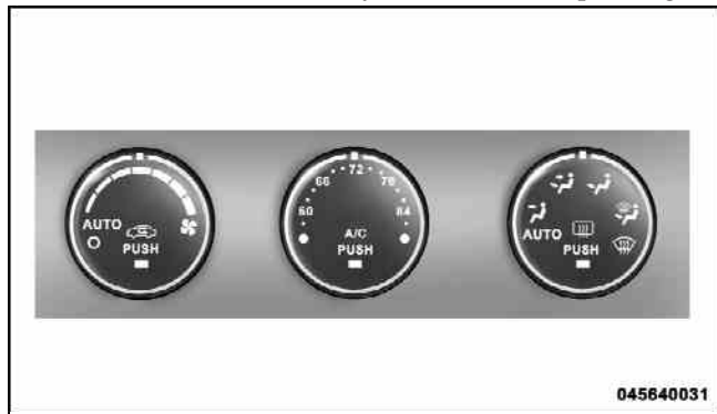
Automatic Temperature Control
